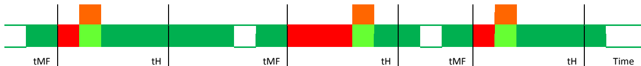
Figure 2.2a. A Series of Brief Outages in Main Power Diminish Energy Stored in the Batteries.
