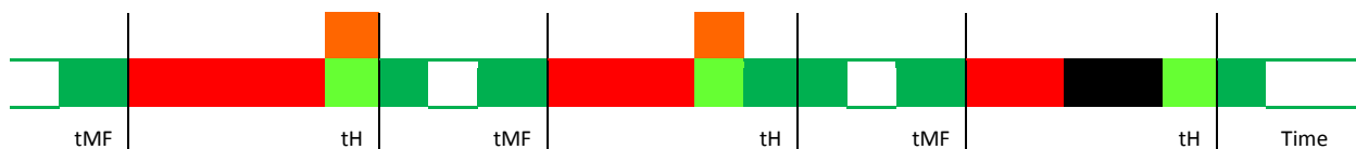
Figure 2.2b. A Series of Brief Outages in Main Power Exhaust the Batteries and an Outage Occurs.
