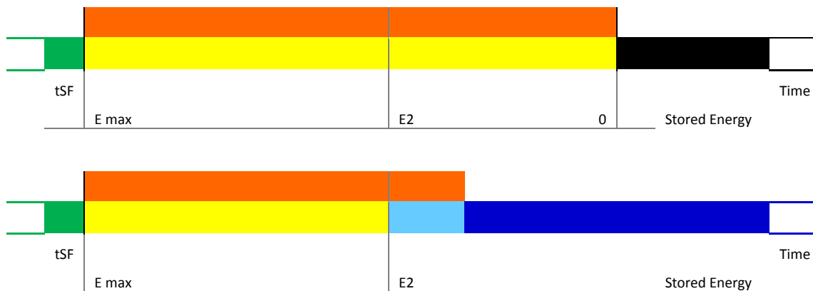
Figure 4. Outcomes of Undetected Failure Condition without (upper) and with (lower) Critical Power Protection Supervisor.
